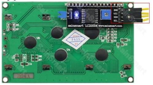
one end of the cable goes to GND, VCC, SDA, SCL, and the other end goes to the corresponding GND, VCC, SDA, SCL on the LCD module.
